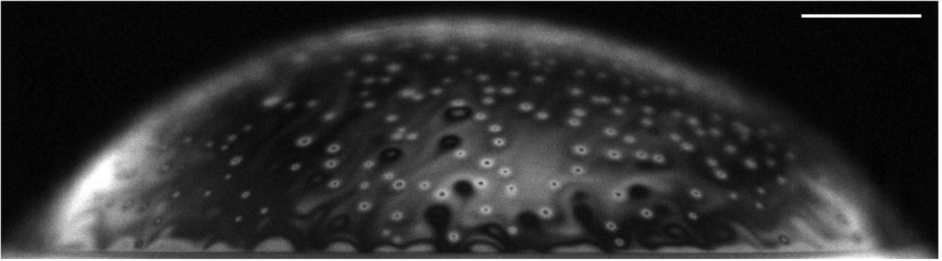
FIG. 2. Fifty second-old bubble observed using monochromatic light (sodium lamp, 589 nm) at the surface of water contaminated with *E. coli*: the bright spots are only observed when bacteria are present and reveal their location and persistence on the cap. Scale bar is 1 mm.
