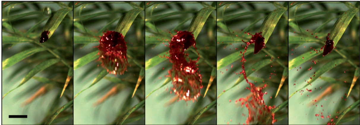
Fig. 4 Splash by raindrop (diameter 5.0 mm, speed 7 m/s) and fragmentation of a contaminated sessile drop on an Areca Palm leaf. We = 3500 and K = 45,000 . The first snapshot is taken at 2 milliseconds prior to the raindrop's impact. Subsequent snapshots at 2, 4, 7, and 11 ms after impact are then displayed. The largest ejected droplet is 1.6 mm in diameter. Scale bar is 1 cm.
