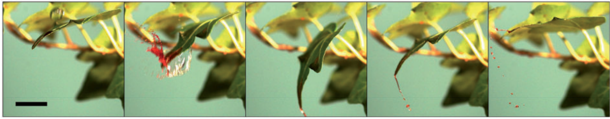
Fig. 6 Coexistence of splash, dripping and catapult during a single impact of a raindrop (diameter 4.6 mm, speed 6.5 m/s) on an English ivy leaf. We = 2780 and K = 35,000 . Snapshots are taken at impact, then 3, 25, 35, and 45 ms later. The largest droplet ejected by splash and detachment are 0.68 and 0.84 mm in diameter, respectively. Scale bar is 1 cm.
